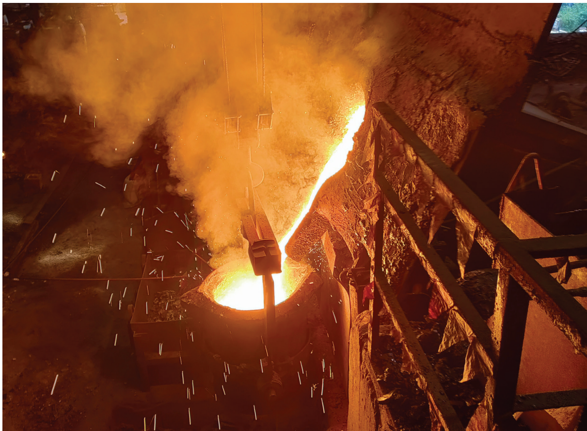
Figure 15: Induction furnace pouring
