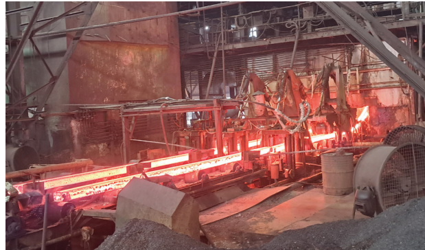
Figure 18: Continuous casting process
